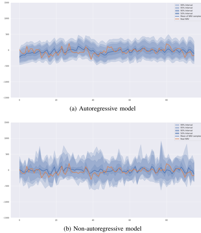
Fig. 2. Comparison between autoregressive and non-autoregressive models. The samples are generated using a linear model using all input features.
